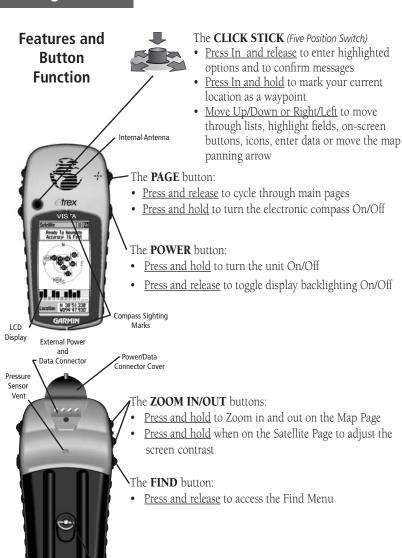
**NOTE:** The eTrex Vista is designed to be held and operated in the left hand, but it can be held and operated using the right hand as well to suit your preference.
