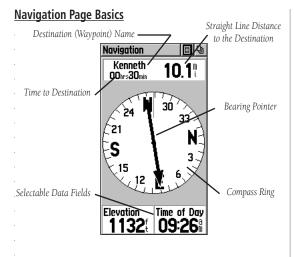
The Navigation Page displays directional information to guide you to a destination. The Status Window at the top of the page shows you the name of your destination, the distance and the time to go. A Bearing Pointer and Compass Ring are displayed to provide you with navigational guidance. Two Data Fields are provided, and can be programmed to display a variety of navigation data.
