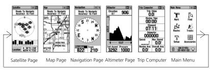
While these six pages provide you with different types of navigation information, they all share common features like Option Menus and a Main Page Menu, both of which are accessed by on-screen buttons. To display these menus, simply highlight the on-screen button and press in on the **CLICK STICK**
