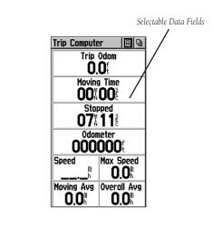
The Trip Computer page displays up to eight different types of navigation data. Each data field is selectable and can contain one of many data information options.
